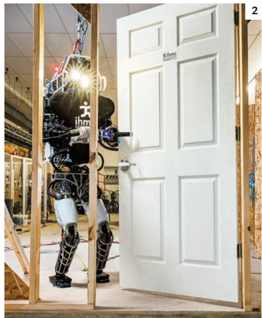
IN ITS CREATORS' laboratory at the Florida Institute for Human & Machine Cognition (IHMC), Running Man climbs stairs (1) and opens a door (2), both tasks from the DARPA Robotics Challenge. John Carff of IHMC guided Running Man through the competition; here he works the lab's control console (3).
